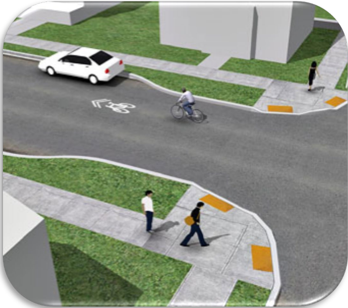
Recommended intersection development consideration for Pine Street and Old Route 66 (south) includes pedestrian bulb-outs like the example designed by the National Association of City Transportation Officials (left) and raised crosswalks and intersections captured by the Federal Highway Association (right)
